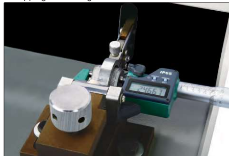
lapping measuring surfaces of outside micrometer
