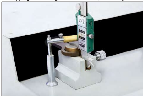
lapping measuring surfaces of caliper lower jaws
